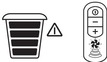
Once the bucket is emptied, simply push one of the two reset buttons located on the power unit and hold for 5 seconds.
