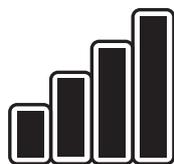
Three to four performance bars indicates the system is performing at the optimal level. Performance levels will change depending on variable speed settings and when specialty cleaning attachments are used. When the unit is OFF, performance bars will display as empty.
